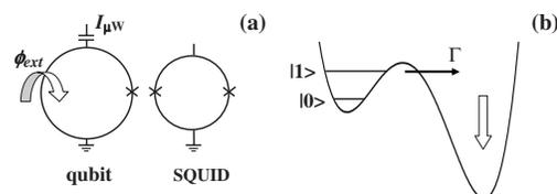
FIG. 1. (a) Schematic of a phase qubit controlled by a microwave current  $I_{\mu W}$  and an external flux  $\phi_{ext}$ , and inductively coupled to a superconducting quantum interference device (SQUID). (b) Lowest energy levels in the left well of the profile  $V(\phi)$  represent the qubit states. Tunneling to the right well from state  $|1\rangle$  is detected by the SQUID.
